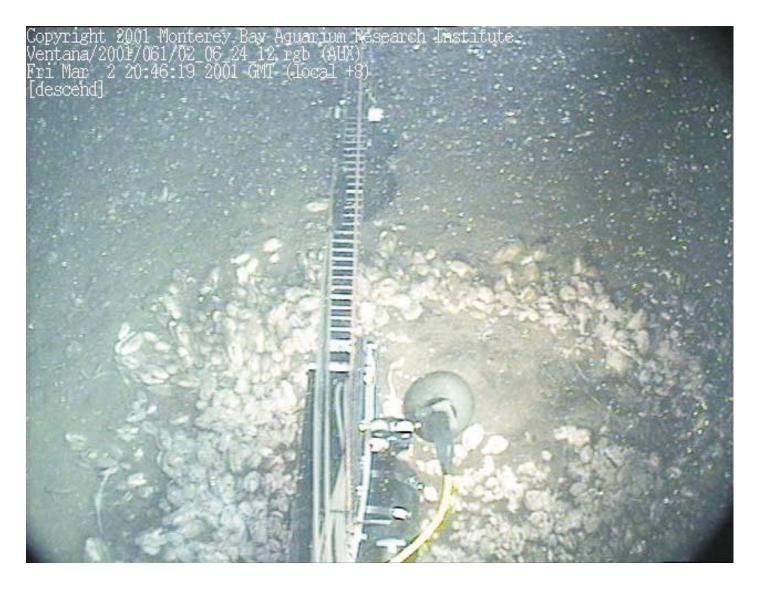
below) revealed that significant concentrations do exist directly over these seeps. The ROV was fitted with a special vertical profiler, built by MBARI personnel, that controlled the height of ISUS above the sediments.
