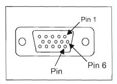
The cable pins are installed by choosing the appropriate conductor color and connector hole location and inserting the pin into the hole until it "clicks" into place. Verify the pin is locked into place by gently pulling on the conductor.
