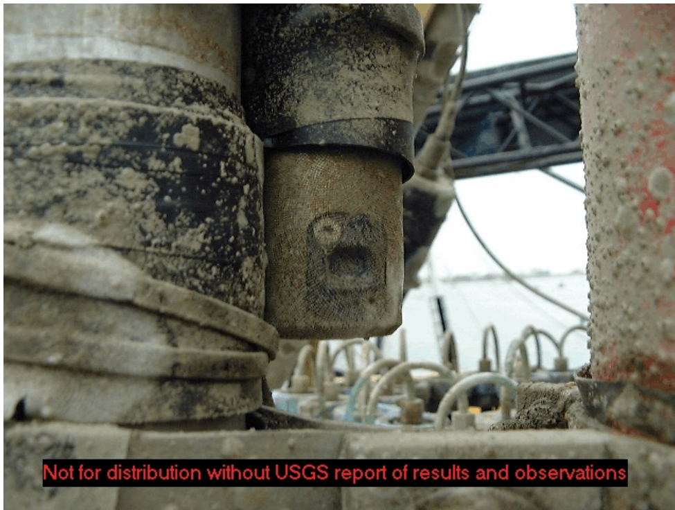
Figure 2: Biofouling on the Aanderaa optode shown as recovered.
